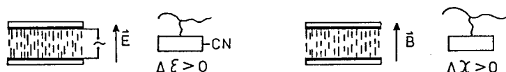
Fig. 3: Macroscopic homeotropic alignment of mesogenic groups in an electric or magnetic field
